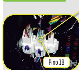
VISÃO SUPERIOR DO CONECTOR CENTRAL ACIMA DA CAIXA DE FUSÍVEL
